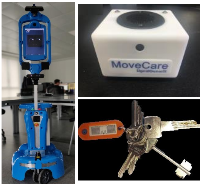
Fig. 2. Giraff.X robot on the left. Notice the two RGB-D cameras above and below the screen and the two RF-ID readers at the basis of the neck. On the right a smart microphone and a tagged object (keys holder) are shown. Notice the eyes blinking on the black screen.
