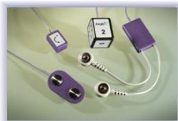
The MyoEX kit uses surface EMG for computerised exercise, biofeedback, muscle re-education. Can be applied to the upper and lower extremities. Uses the electrical activity generated by a muscle contraction to control the set activity in the exercise section. The supplied 'grounding' strap is attached during the testing to combat environmental interference.
