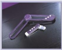
Allows the use of electronic goniometer readings for upper and lower extremity ROM. The kit has a small goniometer for measurement of finger and toes, and a larger goniometer for wrist, elbow, shoulder, hip, knee, and ankle measurements. The interface provides 'live feedback' of measurements taken for each joint, and recordings are taken quickly by the press of a button on the goniometer. The data is then saved to the individual patient file.
